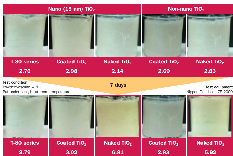
Figure 10: Measurement of the photostability of T-80 compared to 15 nm and non-nano TiO 2 .
