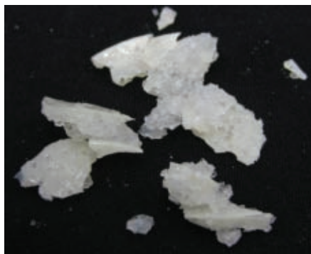
Figure 5: Obtained light material after removing the oil and water of an emulsion. The emulsion was incubated for two weeks at 65 °C in a cabinet dryer.
